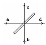
Consider the model of beam-splitter that is sketched in the figure. Light is incident from the a, b input arms and is transmitted/reflected into the c, d output arms. In the classical theory, the beam-splitter operation is summarized by the scattering matrix  $\mathbf{S}(\omega)$  connecting the output fields to the input ones at a given frequency  $\omega$ :
